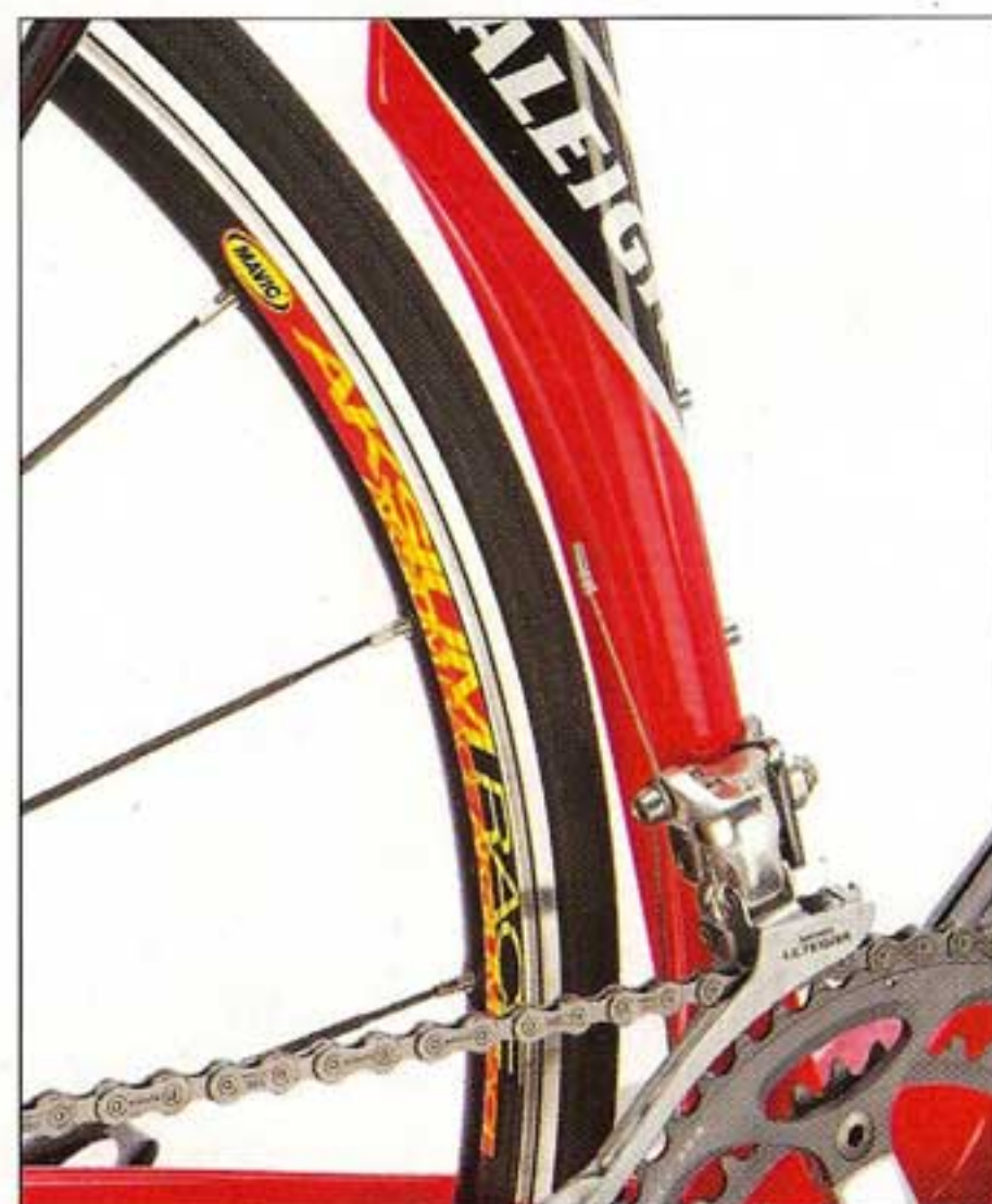
The seat tube arcs around the rear tire, giving the Prestige an aerodynamic and sleek edge.
